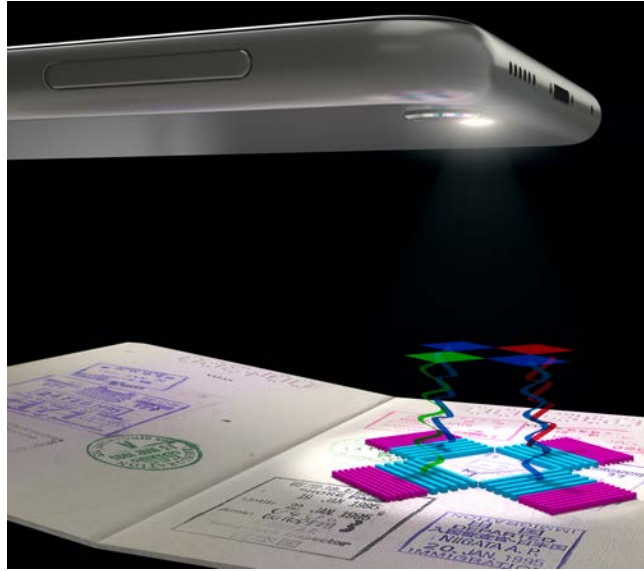
Figure 6: Artist's concept: optical security label made with RWGs that reveals a hidden pattern by using the flash and the camera of a smartphone in a specific spatial position. Image courtesy of Giorgio Quaranta.
